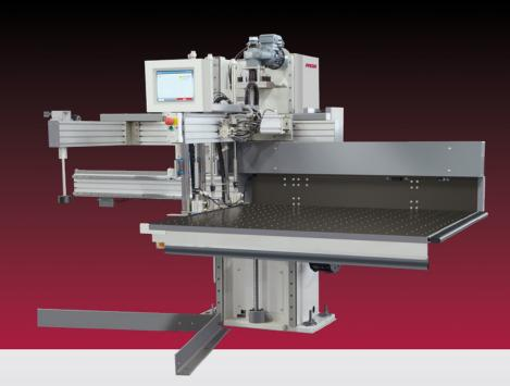
The PRISM Paper Loader is a high-volume, high-production machine built to streamline your cutting process. These heavy duty machines pick up and transport material to the front of the paper cutter. The ergonomic design allows cutting lines to transport sheets faster and more easily. It can be ordered for use on the right or left side of your paper cutter.
