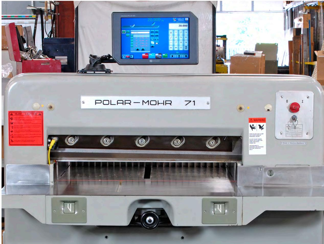
NOTE: The retrofit display is supplied in a small plastic console to facilitate large variations in the mounting. C&P Microsystems does offer an OEM panel for some cutters at an additional cost. Please feel free to contact your dealer, representative, or C&P Microsystems directly for more information.
