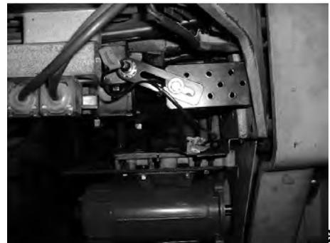
**Clamp Up Sensor** – supplies ground when the clamp is full up.
