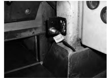
**Clamp Shoe Sensor**—supplies ground to pin 6 when the clamp shoe is in the holder.
