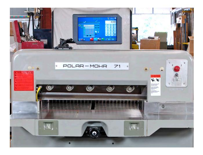
NOTE: The retrofit display is supplied in a small plastic console to facilitate large variations in the mounting. C&P Microsystems does offer an OEM panel for some cutters at an additional cost. Please feel free to contact your dealer, representative, or C&P Microsystems directly for more information.
