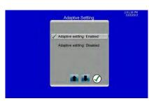
If **ON**, then if the gauge oscillates around the target (a phenomenon known as dither) the tolerances will open slightly to compensate and allow the motor and brake to stabilize. The original tolerances will be reloaded at the next drive command. If **OFF**, then the gauge will continue to
