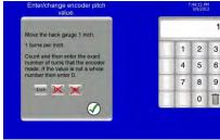
Position the bubble over the Current Pitch Value line. Tap Use to enter the exact number of times the shaft encoder rotates for each inch or cm of gauge movement (see
