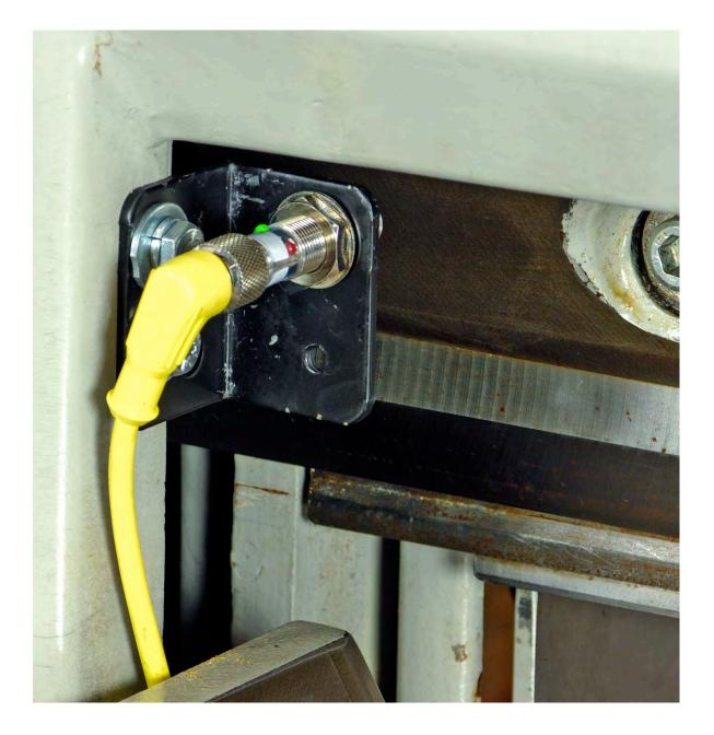
Clamp Shoe Sensor – supplies ground when the clamp shoe is in the holder.
