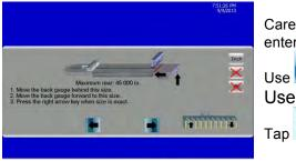
Carefully move the gauge to the Maximum rear position you entered earlier as requested on the screen.
